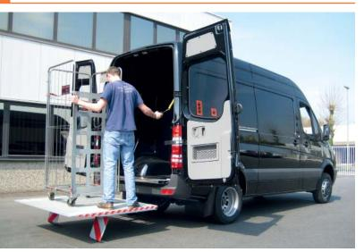
The DH-LSP was the first cantilever lift design, tailor-made to suit factory built panel vans, and DHOLLANDIA still continues to lead the innovations in this field today. Thanks to the **unique shape of the lift arms**, no cut-outs are needed in the vehicle chassis and body, and the **ground clearance** under the lift is maximised.
